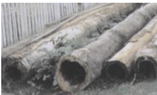
Termite damage in tropical hardwood poles
