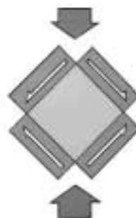
Figure 4 Panel shear schematic based on a test arrangement to create pure tension and pure compression across the diagonals to obtain the shear modulus and ultimate shear strength
