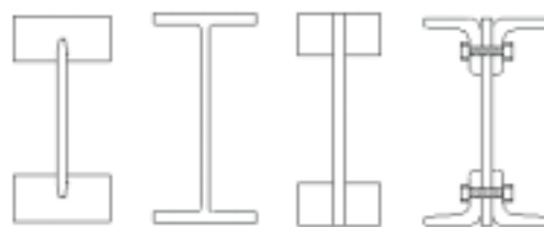
Figure 1 Timber and steel I-joists left: factory produced, right: craft-based
